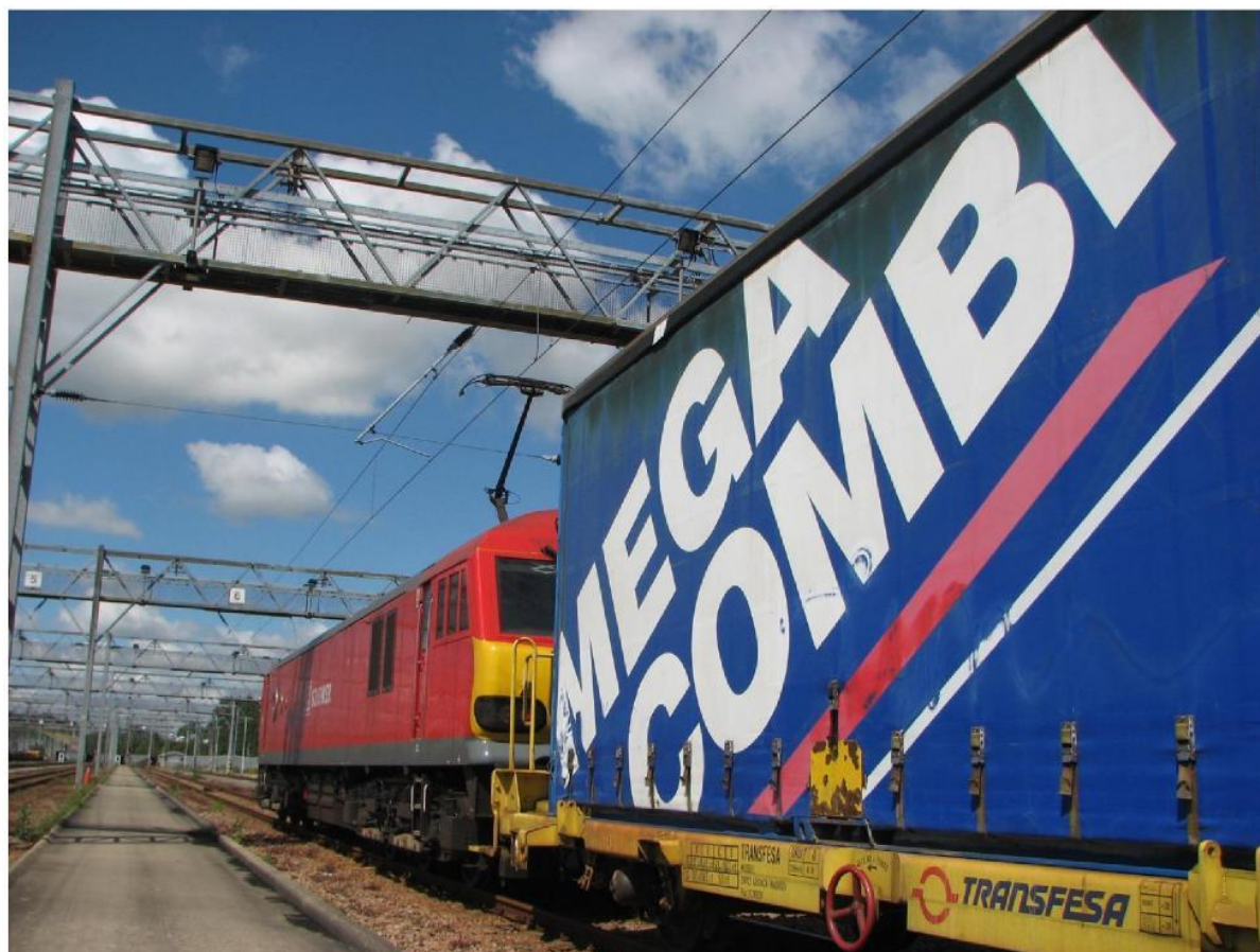
Figure 5.6 Soft sided swap body wagon with bottom lift points
