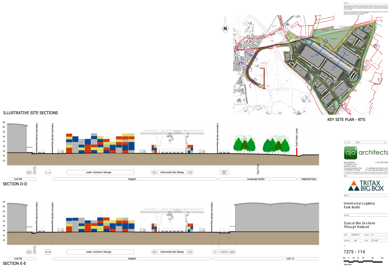
Figure 5.3 A cross section of the Railport
