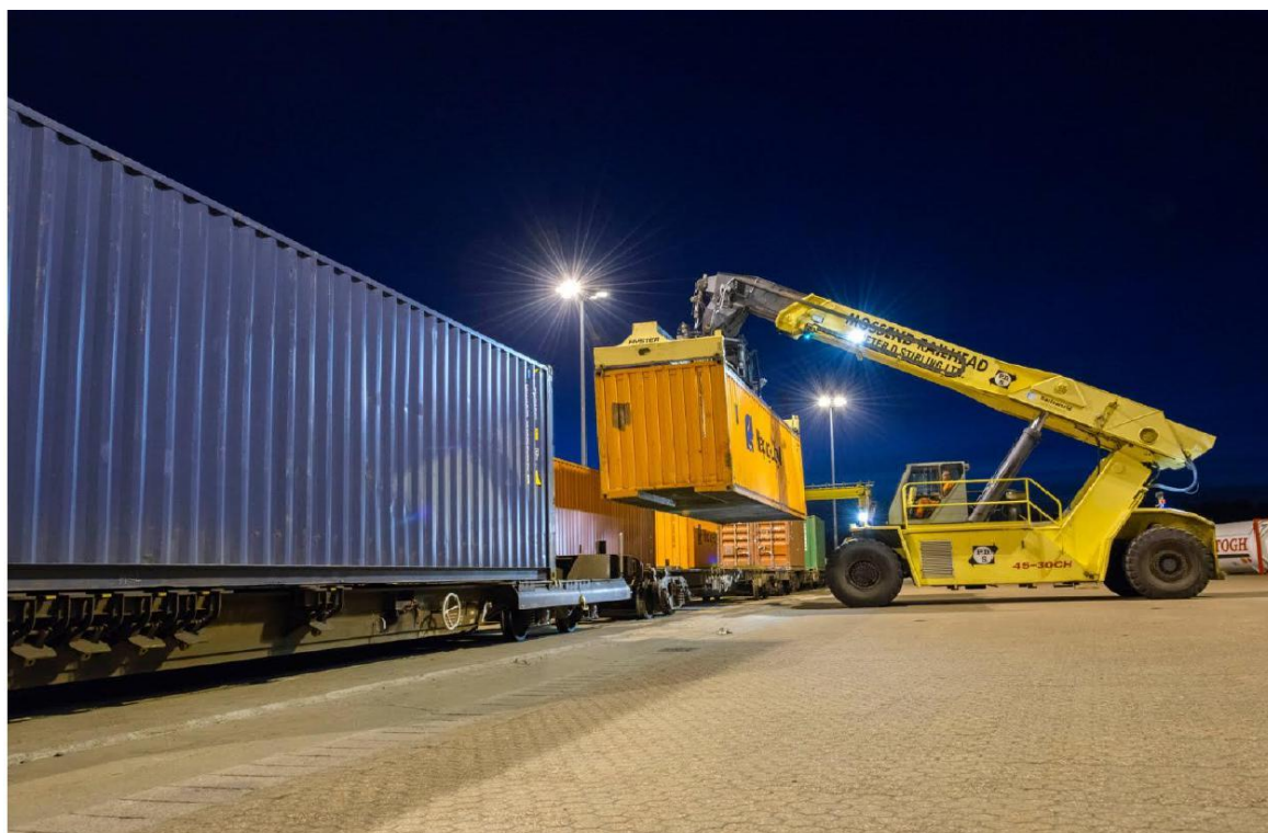
Figure 5.2 A reach stacker in operation
